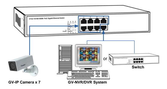
**Note:** The maximum cable length for RJ-45 Cable is 100 meters.
